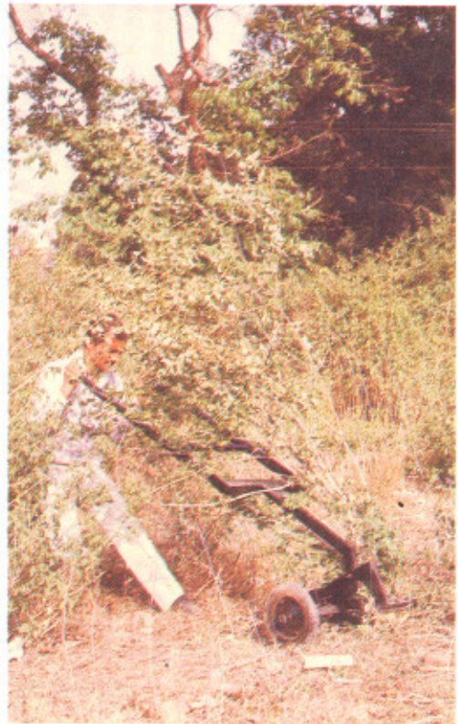
Uprooting of Lantana Bush by Stalk Puller
