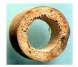
Cross section of bamboo showing damage by *Dinoderus* beetles.
