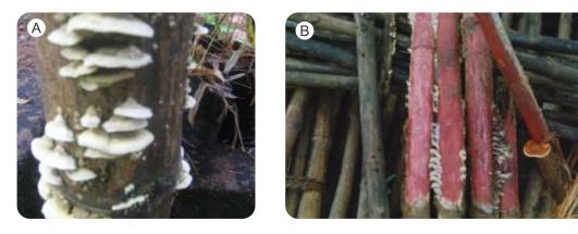
Fig. 9.10: Fungal decay on dried bamboo (A) and in storage (B)
