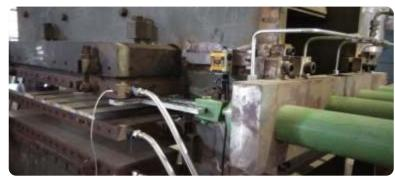
Fig 11.4: Hydraulic hot press with lateral pressing for laminates
