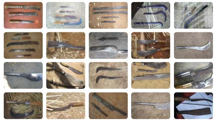
Fig. 11.6: Traditional tools for bamboo working
